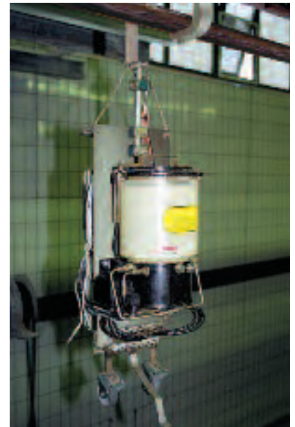
Auto-lubrication system for GERALYN® SGHF2 grease on a monorail conveyor system
